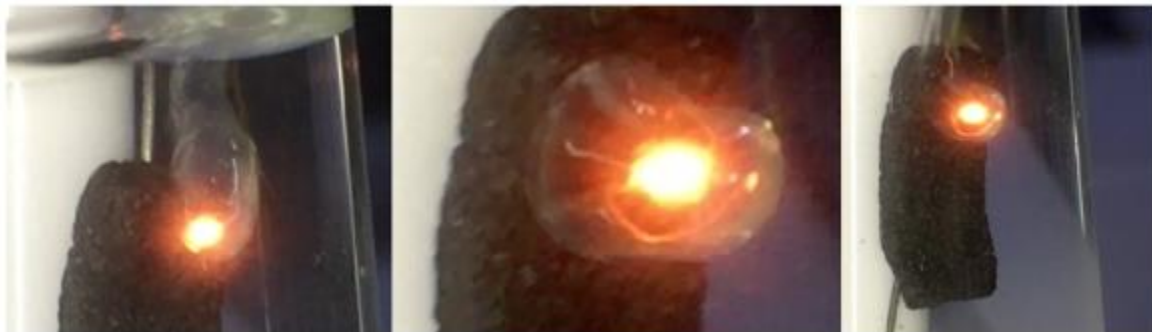
Evolution of a single bubble during continuous laser excitation of graphene aerogel in the methanol
