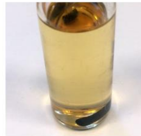
Cuvette of methanol with graphene foam scaffold after irradiation with laser diode 975 nm
