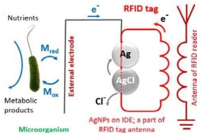
Fig.1. Schematic representation of biosensor-RFID tag for detection of bacterial growth on external electrode.
