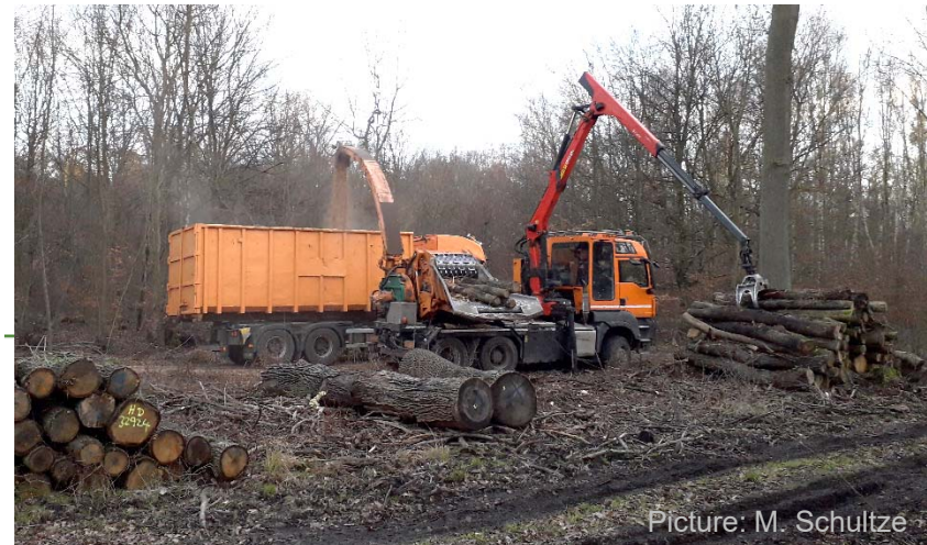
Chipping of logging residues (above) and roundwood (below) into transport vehicle
