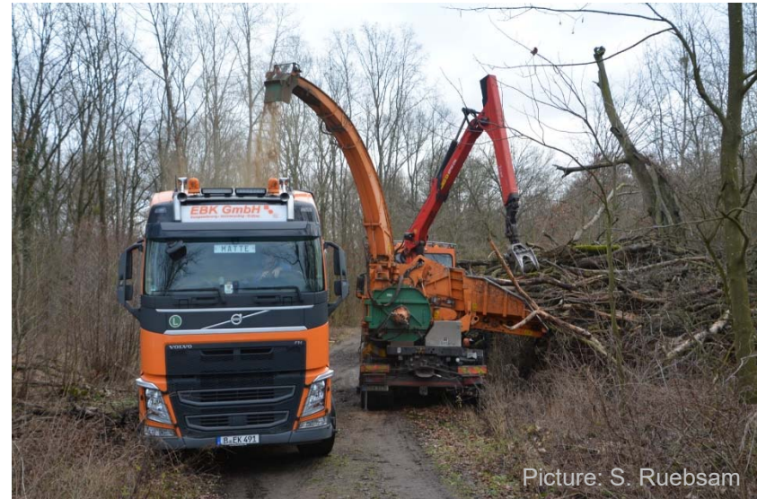
Chipping of logging residues (above) and roundwood (below) into transport vehicle
