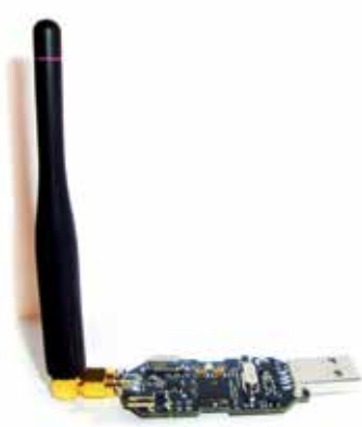
Fig. 3) The OpenBeacon USB1
