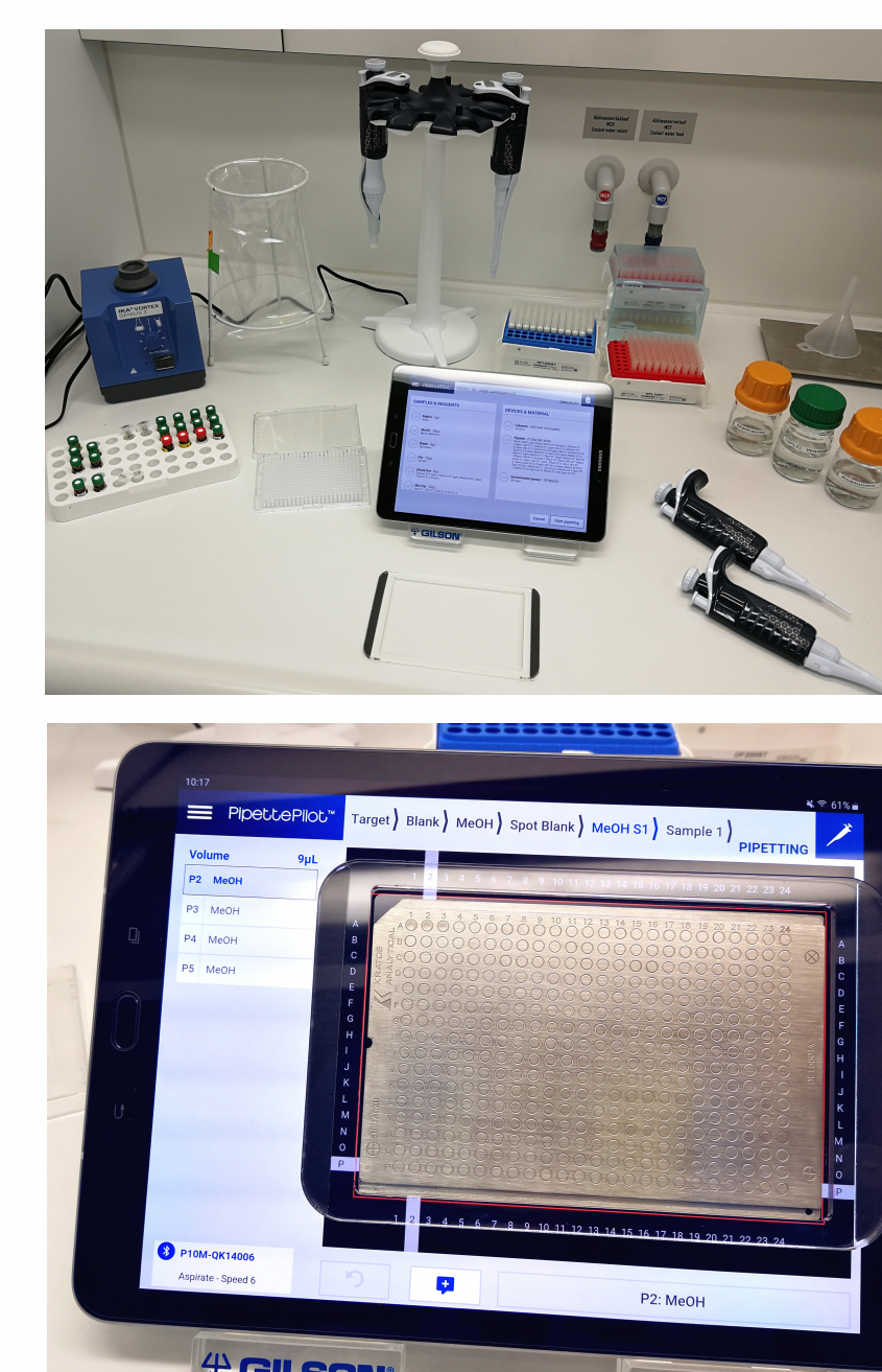
Experimental setup with the Gilson TRACKMAN connected for the MALDI-TOF MS of PACs
